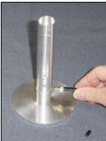
Connecting the cable to the pipette holder.
