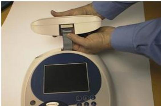
4. Plug the accessory cable into the printer.
