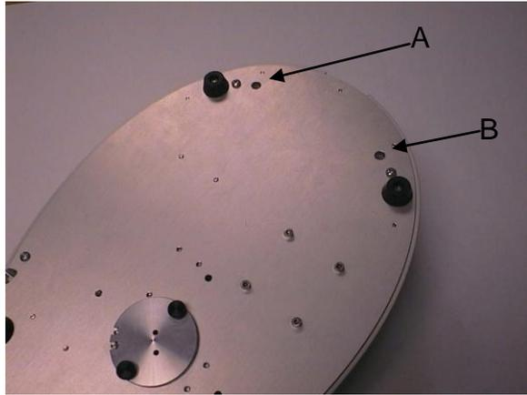
5. Note the slots in the accessory cover, designed to engage with the Bluetooth accessory PCB
