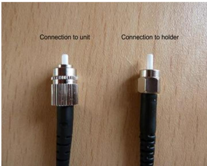
Connect the cables to the base of the pipette holder. Push the connector into the socket and hand-tighten the nut to hold the connector in place. ***Do not use tools to tighten the fixing nut.***
