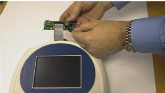
3. Plug the accessory cable into the Bluetooth module.
