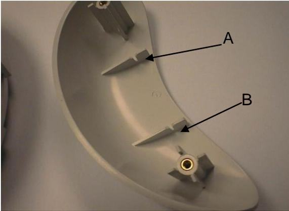
1. REMOVE THE POWER CABLE FROM THE INSTRUMENT. Turn the instrument over and remove the cap head screws from positions A and B using the Allen key provided.
