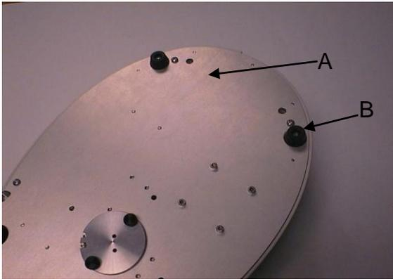
1. REMOVE THE POWER CABLE FROM THE INSTRUMENT. Turn the instrument over and remove cap head screws from positions A and B using the Allen key provided.
