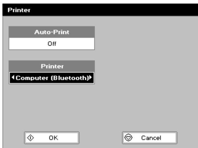
9. Switch the instrument on and go to the preferences page under utilities/instrument, and select the Bluetooth option.
