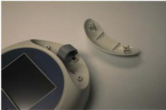
2. Turn the instrument back over and lift the accessory cover vertically upwards to remove. Remove the tie-wrap from the cable.
