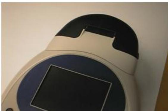
5. Lower the printer onto the locating bosses and push down firmly.
