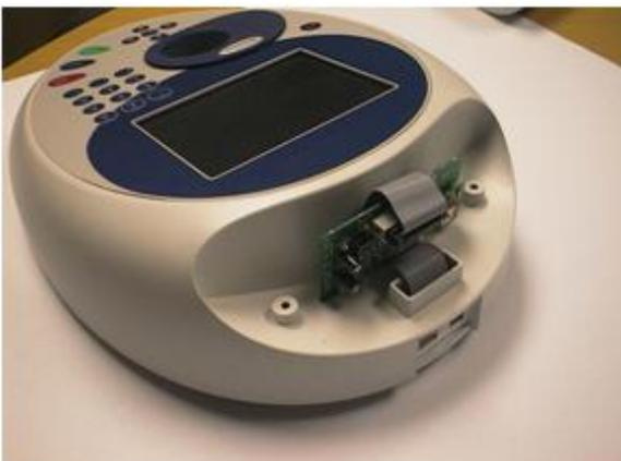
4. Note the slots in the base of the case. The two lugs on the Bluetooth module plug into these
