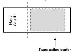
**IMPORTANT!** Do not mount more than one section per slide. Place sections in the center of the slide.
