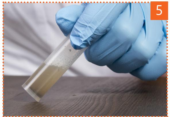
■ Tap the sample tube on a hard surface so that all the liquid is collected at the bottom of the tube.
