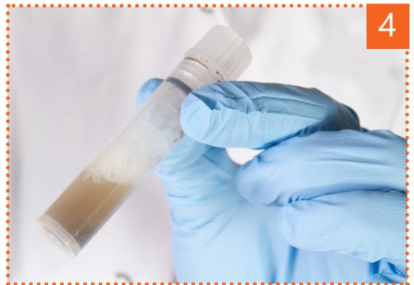
■ Shake the sample tube to homogenize well.
