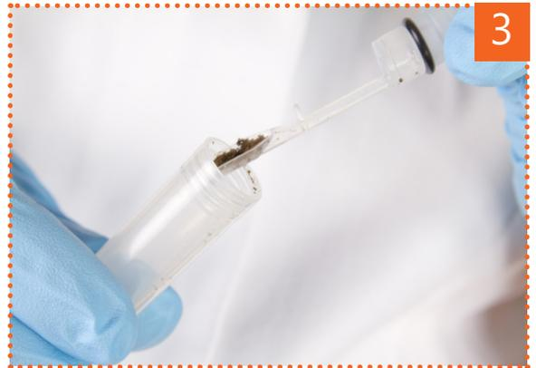
■ Dilute its content in the liquid of the small tube called sample tube.
