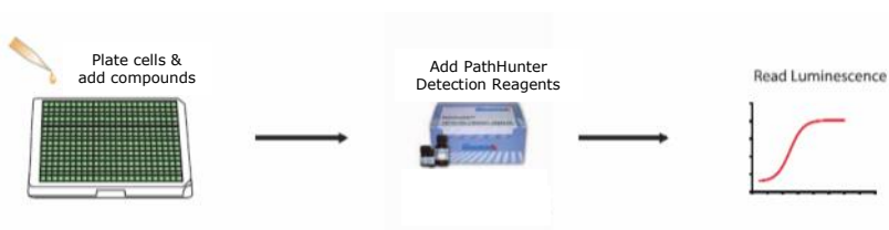
Figure 4. Simple chemiluminescent assay protocol for monitoring GPCR activity in response to compound challenge.
