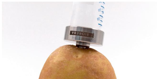
**BIOpick** is a device for taking heel core samples from potato tubers (e.g. for testing for quarantine bacterial diseases such as ring rot caused by *Clavibacter* and brown rot caused by *Ralstonia*). It makes coring more ergonomic and allows up to 200 heel end cores to be collected and transferred into a 50ml collection tube. Sampling can be performed manually or semi-automatically by connecting the BIOpick to a laboratory blender using the supplied adapter.
